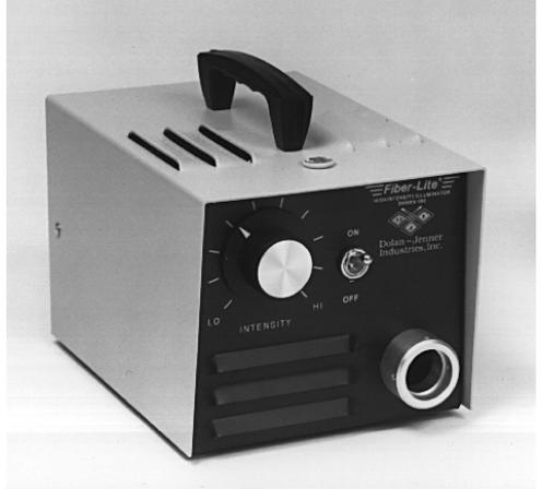
Model 180 and 170-D Illuminators are readily interchangeable within the systems. The exceptions are with System 181, 181A and 181B which require the Model 180 Illuminator for the support of the self-supporting fiber optic light pipes EEG 2823, EEG 3922 and BG 2820. In addition the Model 180 has the lowest noise and vibration characteristics that can be incorporated into any unit, which makes it especially suitable for high magnification stereo-microscope usage.
